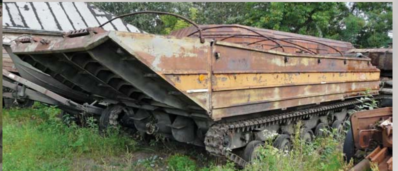
Below & bottom: two views of the K-61 showing full length of this long narrow vehicle. This amphibian when in the water and fully laden became very unstable.
